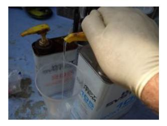
The west systems epoxy pumps deliver the right proportion of resin to hardener, which is critical to a good repair. If the proportion is off, the epoxy won't harden.
