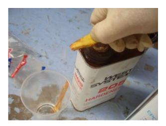
One squirt of resin, and one squirt of hardener provides about two tablespoonfuls of mixed resin/hardener, which is way more than enough for a ding repair.
