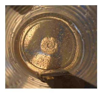
When the resin and hardener are mixed, there won't be any streaks. For best results, keep mixing for another minute or so, to be absolutely sure the resin and hardener are thoroughly mixed.
