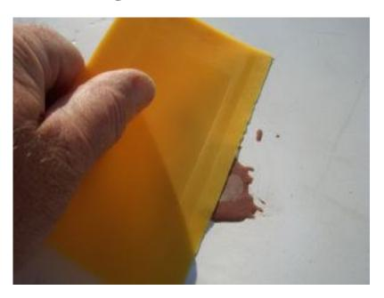
Force the resin/hardener/filler mix into the ding with a yellow plastic squeegee. Once the ding is filled, use the squeegee to level off the top of the mix, leaving a smooth surface.
