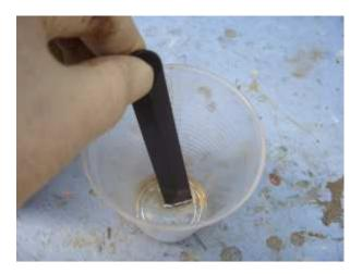
The resin and hardener need to be very, very thoroughly mixed or they won't react completely, which gives a gooey result that has to be scraped off.
