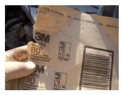
Find a sheet of clean sandpaper. This is 80 grit, which will sand the board's surface to a very rough texture, which is better for the repair.
