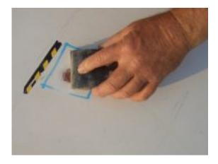
When the epoxy is fully hardened, use a sanding block and sand paper to sand the epoxy flat and level with the surface of the board.
