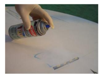
The final step is to spray paint the sanded epoxy. The paint protects the cured epoxy from UV, which will break down the epoxy if it's not shielded from the sun.
