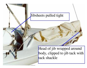
In higher winds, jib handling is hard when you're single-handing. It's probably best to lower the jib and sail on just a reefed main. To lower and secure the jib while out sailing, anchor or capsize, lower the jib, and detach and stow the halyard. The jib can be secured on deck by 1) trimming both jibsheets, and securing them to the cleats nearest the blocks and 2) undoing the top jib hank from the forestay,
