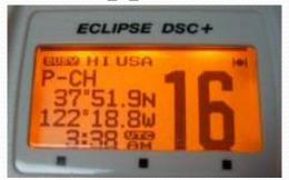
When first turned on, some GPS receivers display the last known position until a new fix is obtained. This position does not get sent to the radio, so the radio will not show the position until the fix is updated.
