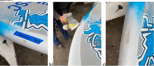
Figure 1. Sanding down a damaged area a) initial dent. b) sanding with a rotary sander. c) the damaged area after sanding
