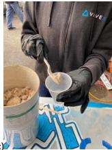
Figure 5. Adding filler to the epoxy to increase viscosity a) split your dose of epoxy to have some pure epoxy later on. b) The filler is in the closet. c) Progressively add filler to the epoxy until you get a viscosity close to peanut butter
