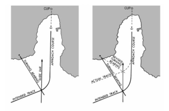
Figure 801c. The slide bar technique.
