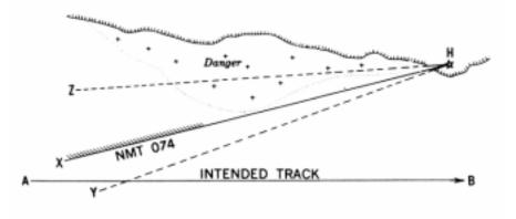
Figure 801d. A danger bearing, hatched on the dangerous side and labeled wih the appropriate bearing.
