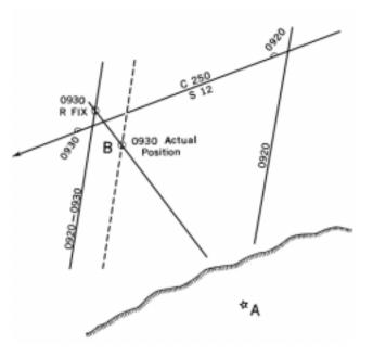
Figure 820a. Effect of a head current on a running fix.
