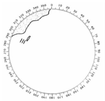
Figure 1308b. Coded racon signal.
