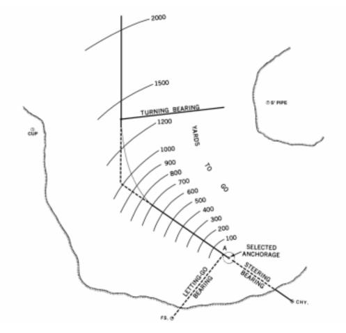
Figure 817. Anchoring.
