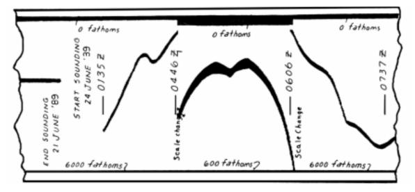
Figure 3016a. Properly annotated echo sounding record.
