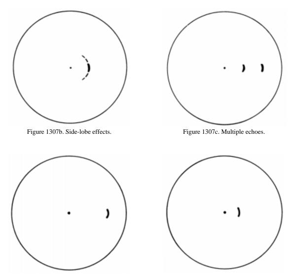
Figure 1307d. Second-trace echo on 12-mile range scale.
