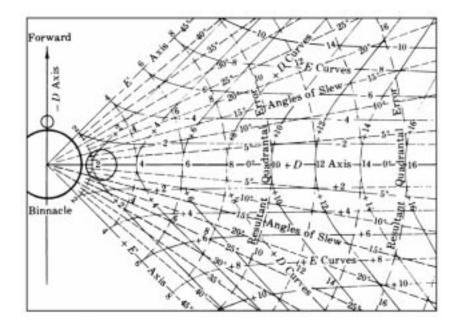
Figure 620. Slewing of quandrantal spheres.
