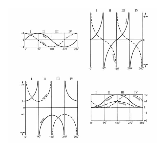
Figure 2109b. Graphic representation of values of trionometric functions in various quadrants.
