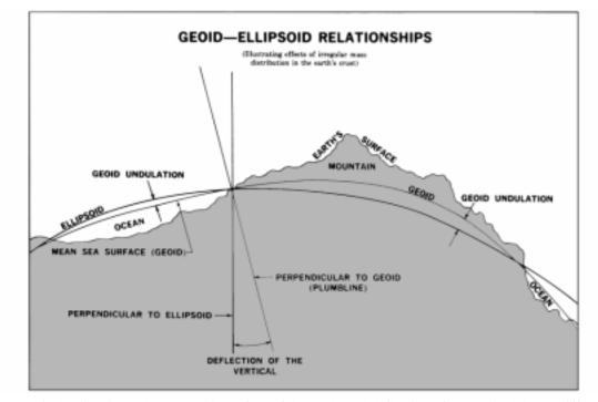
Figure 201. Geiod, ellipsoid, and topographic surface of the earth, and deflection of the vertical due to differences in mass.
