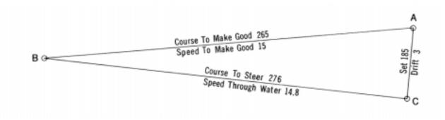
Figure 708c. Finding course to steer and speed to use to make good a given course and speed through the current.
