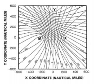
Figure 1206b. A hyperbolic lattice formed by station pairs M-X and M-Y.
