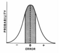
Figure 2302. Normal curve of random error with 50 percent of area shaded. Limits of shaded area indicate probable error.
