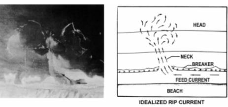
Figure 3319. A rip current (left) and a diagram of its parts (right). Courtesy of Robert L. Wiegel, Council on Wave Research, University of California.
