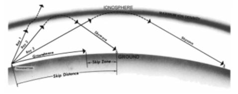
Figure 1007a. The effect of the ionosphere on radio waves.
