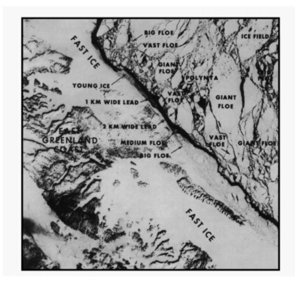
Figure 3412b. Example of satellite imagery with a resolution of 80 meters.
