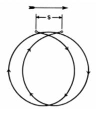
Figure 3303. Orbital motion and displacement, s, of a particle on the surface of deep water during two wave periods.
