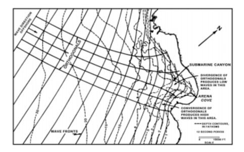
Figure 3316. The effect of bottom topography in causing wave convergence and wave divergence. Courtesy of Robert L. Wiegel, Council on Wave Research, University of Californiia.
