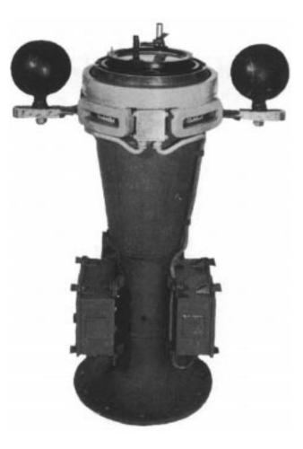
Figure 646. Type K degaussing compensation installation.
