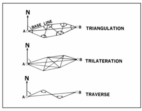
Figure 206. Triangulation, trilateration, and traverse.
