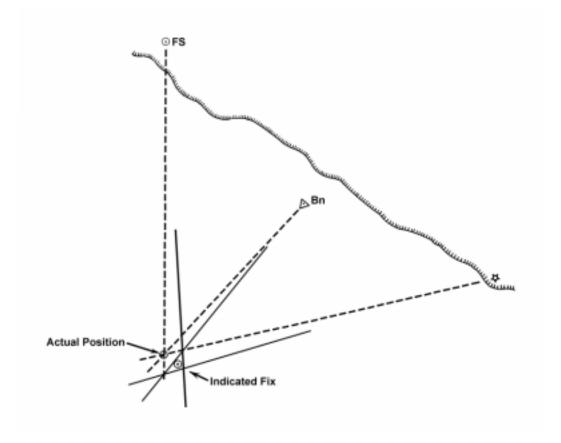
Figure 825. Adjusting a fix for constant error.
