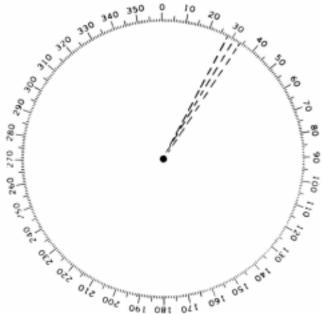
Figure 1308c. Ramark signal appearing as a broken radial line.
