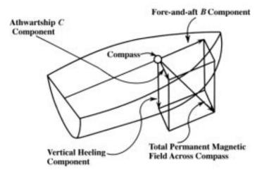
Figure 605a. Components of permanent magnetic field.
