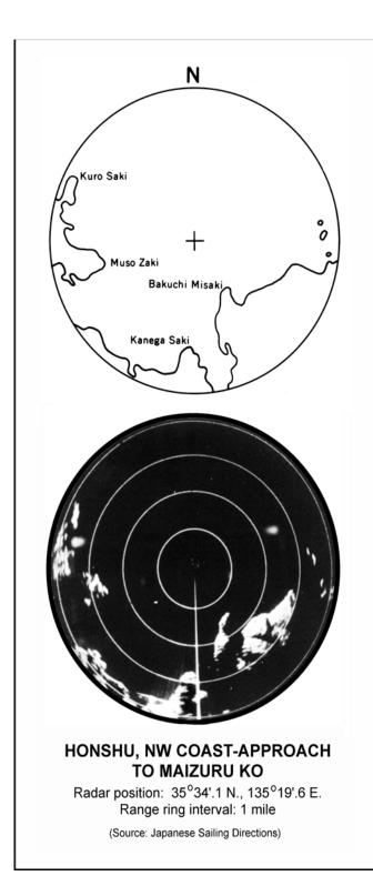
Figure 1302. Plan Position Indicator (PPI) display.
