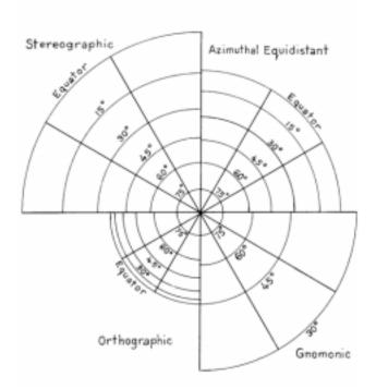
Figure 320. Expansion of polar azimuthal projections.
