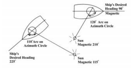
Figure 630. Azimuth circle set-ups.
