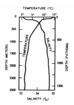
Figure 3110a. Typical variation of temperature and salinity with depth for a mid-latitude location.
