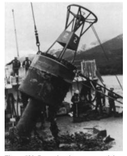
Figure 509. Buoy showing counterweight.
