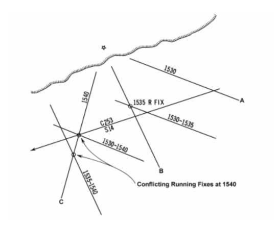
Figure 821a. Detecting the existence of an oblique current, by a series of running fixes.
