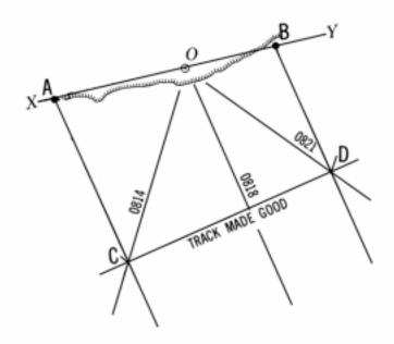
Figure 821b. Determining the track made good.
