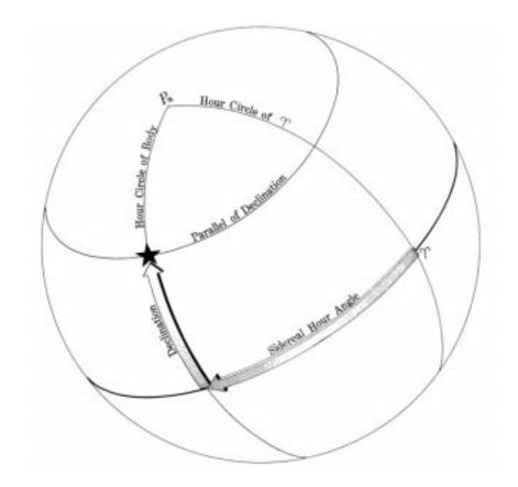
Figure 1524b. A point on the celestial sphere can be located by its declination and sidereal hour angle.
