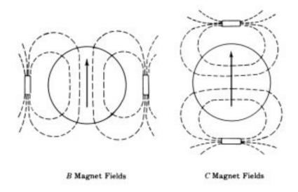
Figure 626b. Arrangements of corrector magnets.
