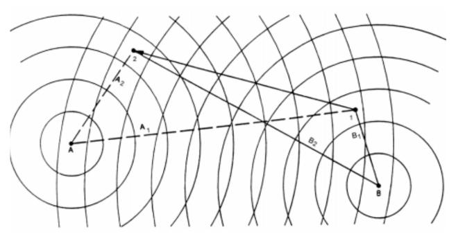
Figure 1213b. Position fixing in the direct ranging mode.
