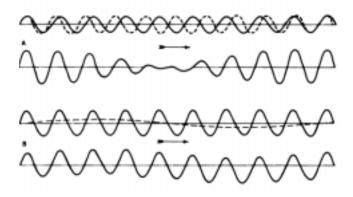
Figure 3302c. Interference. The upper part of A shows two waves of equal height and nearly equal length traveling in the same direction. The lower part of A shows the resulting wave pattern. In B similar information is shown for short waves and long swell.
