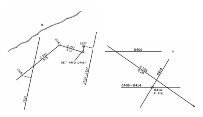
Figure 813d. Advancing a line of position by its relation to the dead reckoning.
