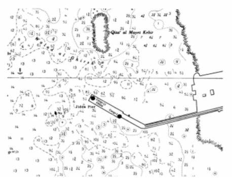
Figure 326b. Part of a nautical chart made from the boat sheet of Figure 326a. Compare the number of soundings in the two figures.
