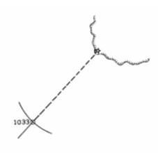
Figure 811d. A fix by range and bearing of a single object.
