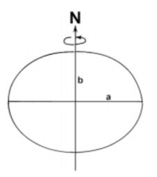
Figure 202. An ellipsoid of revolution, with semimajor axis (a), and semiminor axis (b).
