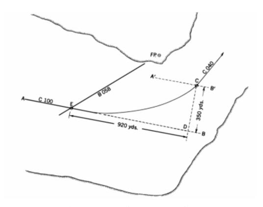
Figure 801b. Allowing for advance and transfer.
