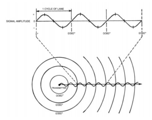
Figure 1213a. Omega lanes formed by radio waves.
