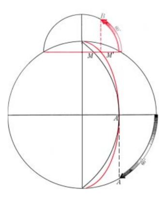
Figure 1529f. Locating a point on an ellipse of a diagram on the plane of the celestial meridian.
