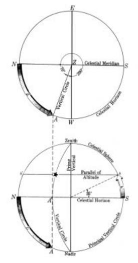
Figure 1529b. Measurement of horizon system of coordinates.
