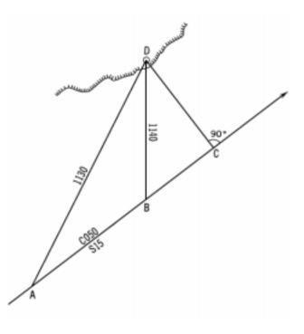
Figure 822. Triangles involved in a Table 18 running fix.
