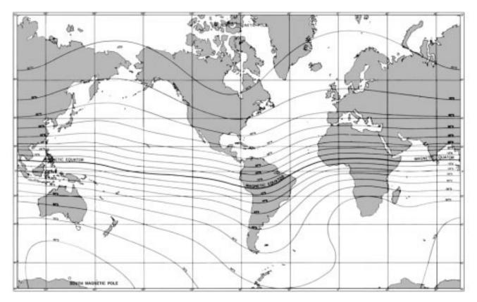
Figure 603b. Magnetic dip chart, a simplification of chart 30.
