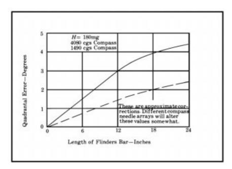
Figure 622. Quadrantal error from standard Navy Flinders bar.
