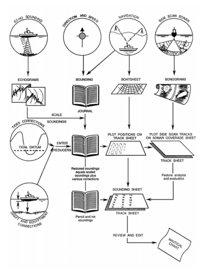
Figure 3004. The process of hydrographic surveying.
