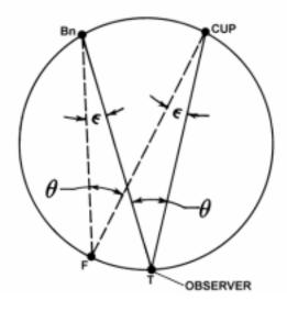
Figure 824a. Two-bearing plot.
