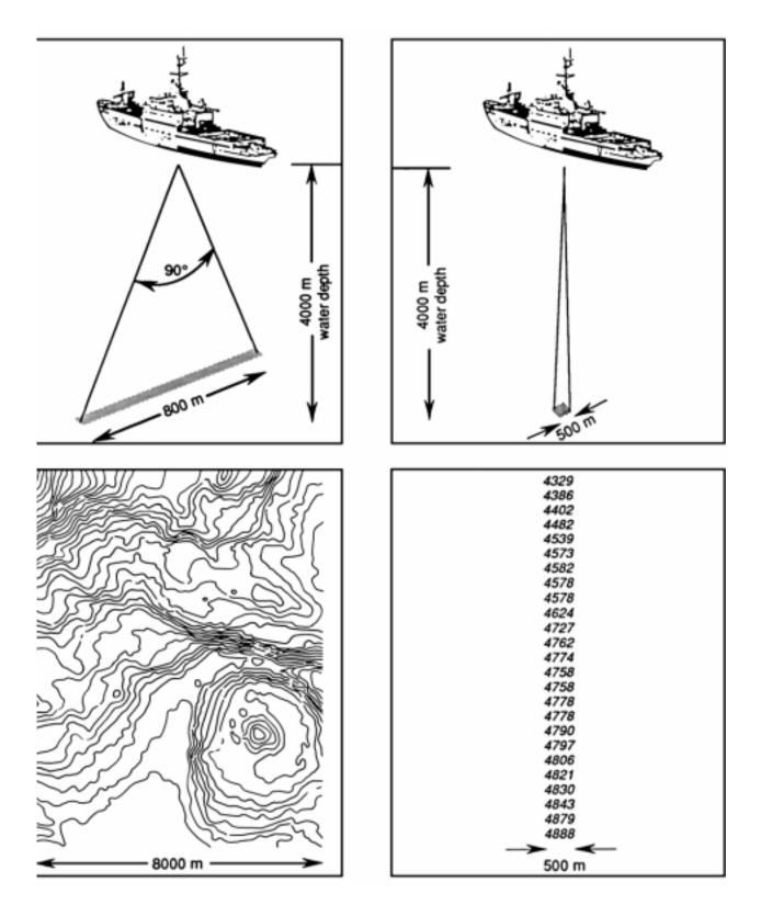
Figure 3005. Swath versus single-transducer surveys.
