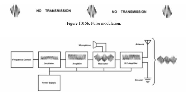
Figure 1016. Components of a radio transmitter.
