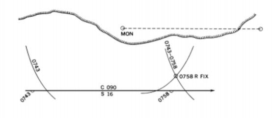
Figure 813g. A running fix by two circles of position.
