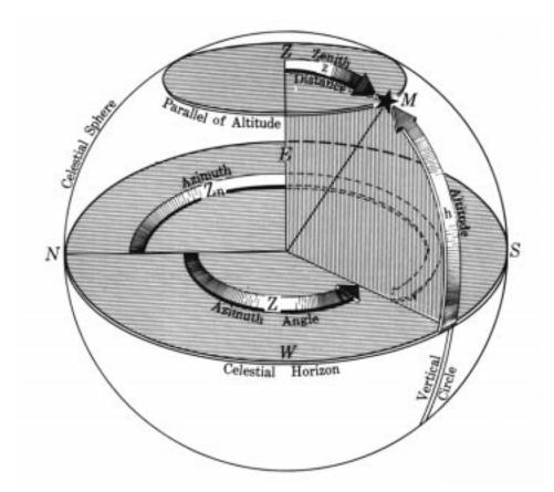
Figure 1527b. The horizon system of coordinates, showing measurement of altitude, zenith distance, azimuth, and azimuth angle.
