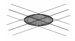
Figure 2304b. Ellipse of uncertainty with lines of positions of equal probable errors crossing at an oblique angle.
