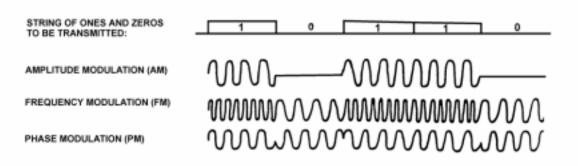
Figure 1106a. Digital data transmission with amplitude, frequency and phase modulation.
