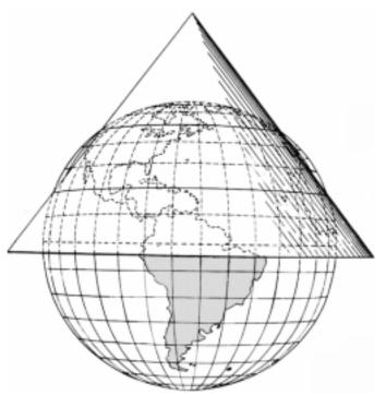
Figure 313. A secant cone for a conic projection with two standard parallels.
