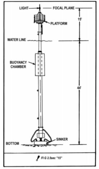
Figure 501b. Typical design for a buoyant beacon.
