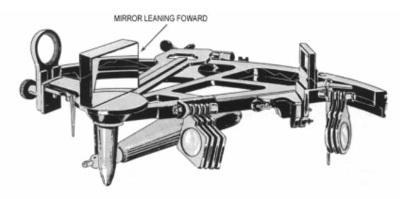
Figure 1612a. Testing the perpendicularity of the index mirror. Here the mirror is not perpendicular.
