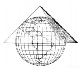
Figure 312a. A simple conic projection.
