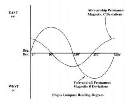
Figure 605b. Permanent magnetic deviation effects.
