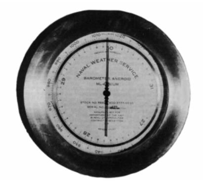
Figure 3703. An aneroid barometer.
