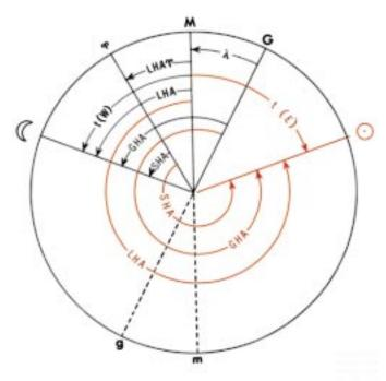
Figure 1525b. Time diagram. Local hour angle, Greenwich hour angle, and sidereal hour angle are measured westward through  $360^{\circ}$ . Meridian angle is measured eastward or westward through  $180^{\circ}$  and labeled E or W to indicate the direction of measurement.
