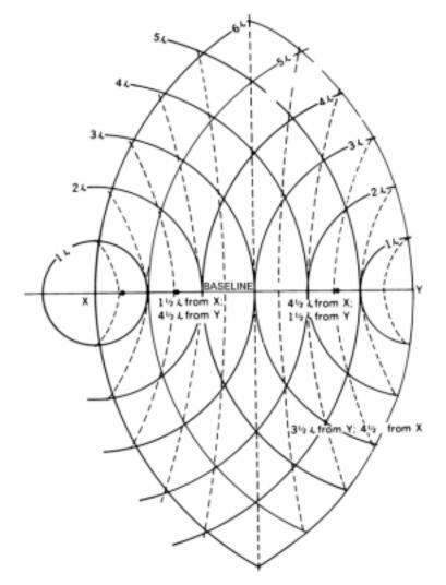
Figure 1214. Omega lanes formed by hyperbolic isophase contours.
