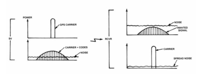
Figure 1106c. GPS signal spreading and recovery from satellite to receiver.
