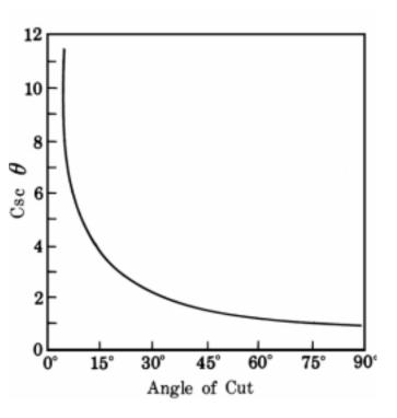
Figure 824c. Error of two-bearing plot.
