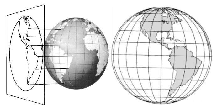
Figure 318a. An equatorial orthographic projection.
