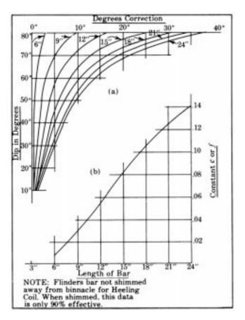
Figure 624a. Dip deviation curves for Flinders bar.
