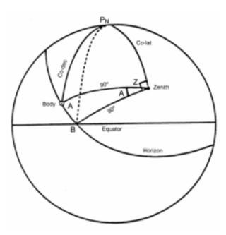
Figure 1703. The amplitude is the arc (A) between the observed body on the horizon and the point where the observer's horizon intersects the celestial equator.
