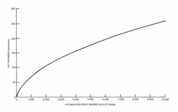
Figure 3404b. Relationship between accumlated frost degree days (°C) and ice thickness (cm).
