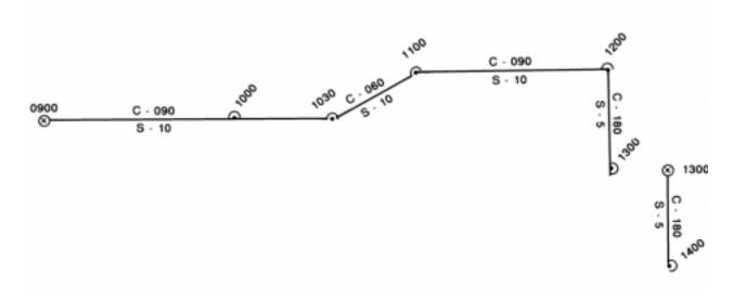
Figure 703. A typical dead reckoning plot.
