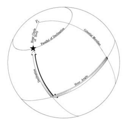
Figure 1524c. A point on the celestial sphere can be located by its declination and hour angle.
