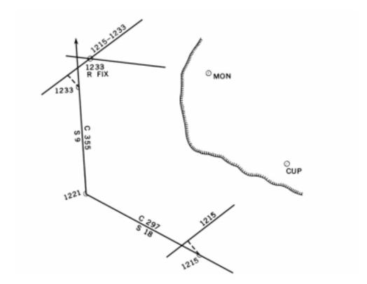
Figure 813f. A running fix with a change of course and speed between observations on separate landmarks.
