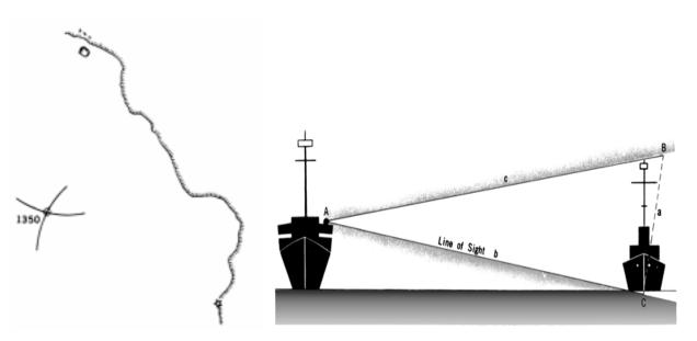
Figure 811b. A fix by two radar ranges.
