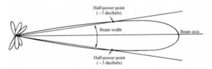
Figure1303b. Radiation diagram.
