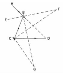
Figure 1601. Optical principle of the marine sextant.
