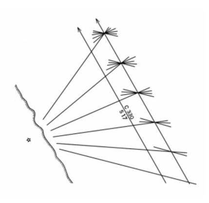
Figure 820b. A number of running fixes with a following current.
