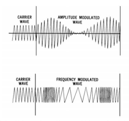
Figure 1015a. Amplitude modulation (upper figure) and frequency modulation (lower figure) by the same modulating wave.
