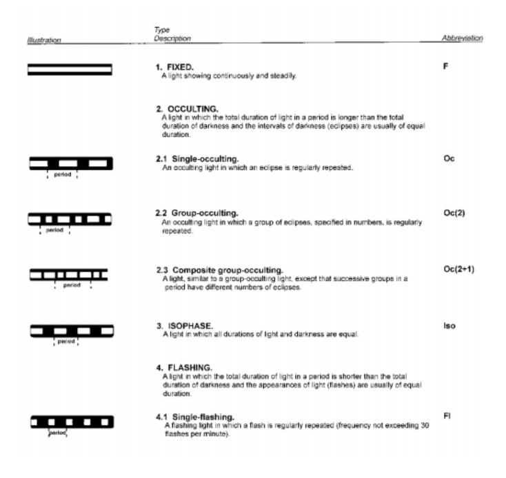
Figure 506a. Light phase characteristics. = = = = = THIS FIGURE HAS TO BE REPAIRED!! = = = = = =
