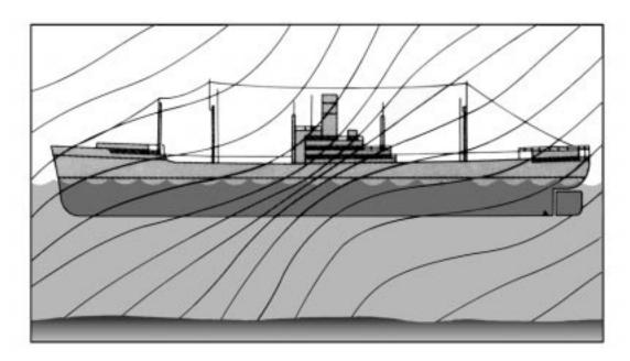
Figure 641a. Simplified diagram of distortion of earth's magnetic field in the vicinity of a steel vessel.
