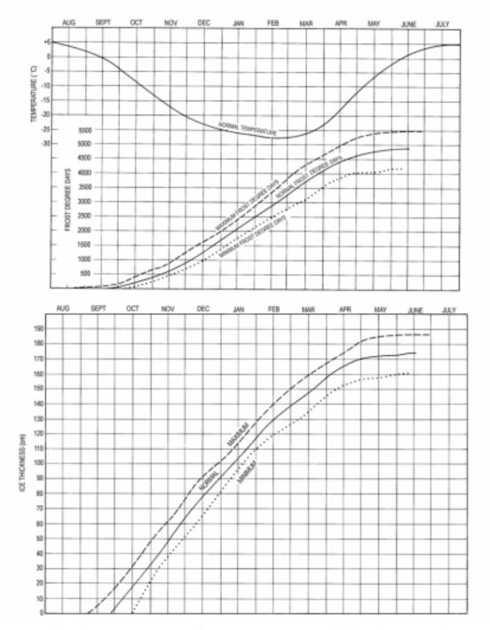
Figure 3404a. Relationship between accumulated frost degree days and theoretical ice thickness at Point Barrow, Alaska.
