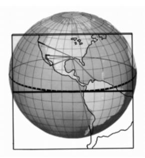
Figure 317a. An equatorial stereographic projection.
