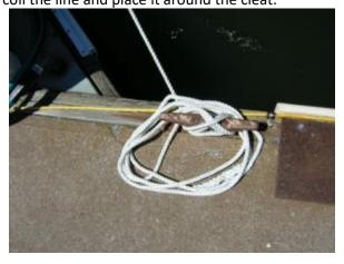
Why: A jumble of line creates a tripping hazard. The lines can get kicked into the water, and they can get stepped on, too, which is not good for the line.
