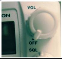
Why: Leaving the radio on will shorten the life of the display. If you forget to plug in the power cord, the radio will run down the battery. If you had the squelch on an the volume turned up loud, live-aboards nearby may be awakened in the middle of the night by radio traffic.
