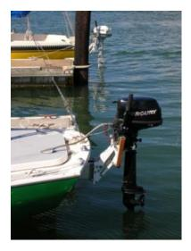
Do: Tilt the motor to the first position (**not all the way up**) on your boat **and** any of the surrounding boats whose motors you may have tipped down before you went sailing. The bottom end should clear the water by an inch or two.
