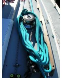
Why: The lines are often wet, especially if you rinse off the boat after sailing, and they tend to stay wet for a long time if they are bunched up. If lines are in close contact with the wood, the wood absorbs water and stays moist, which promotes rot (note the dark spots on the handrail where this halyard was tied).
