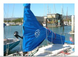
Why: Leaving the cover open allows it to luff in the breeze, which can damage the cover and leave the sail uncovered. If you find it difficult to close the bottom buckle at the mast, **ease the boom lift**.
