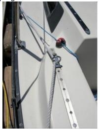
Do: Use the excess bow and stern lines as aft and forward spring lines. They can be tied to the shroud turnbuckles or the winches (or the stanchions, as long as they are tied close to the deck).
