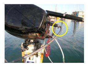
Do: Make sure that the motor is positioned so that there is some slack in the fuel line.
