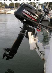
Why: Some of the motors will sit partly in the water when tilted down, even if the mount is raised. Immersion allows marine life to form and, more importantly, promotes corrosion.
