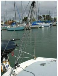
Why: Constant backstay tension puts strain on the mast and rigging, and they can develop a permanent set.
