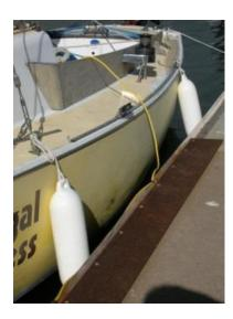
Do: Hang the fenders near the widest part of the hull – usually from the winch and the shrouds.
