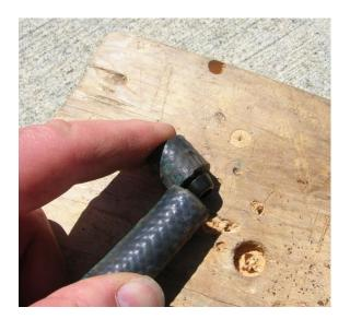
Insert the barbed tube on the connector into the hose. Some twisting may be needed, but be careful not to break the connector. Wiping a little kerosene on the barbed tube will lubricate it and allow it to slide more easily into the hose (a bottle of kerosene is kept in the dock box).
