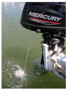
If water is coming out but not in one, steady stream, insert a piece of wire or a pipe cleaner an inch or two into the hole to clear salt or debris that may be interfering with the flow of water. See the pictures below for the location of the hole.
