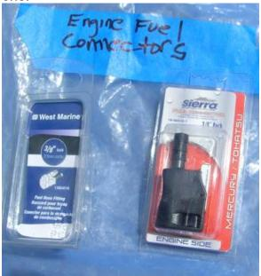
You will need a knife to cut the end of the fuel line and a screwdriver to loosen the hose clamp. There are pieces of wood in some of the dock boxes and parts of the dock that can be used for a cutting surface (DO NOT USE THE BOAT FOR A CUTTING SURFACE). It is recommended that you disconnect the adapter section from the fuel line and work on the dock since there will likely be some gasoline remaining in the line that will leak out.
